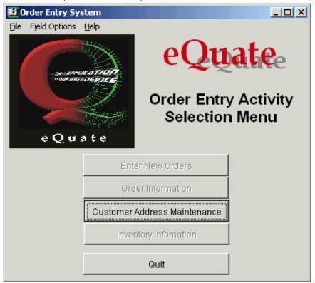
The ECMSTART form will be initially displayed when the user selects the corresponding eQuate Application from the eQuate Session Manager; however, the COBOL program will call for this form to be re-displayed whenever the user presses the Exit button on the ECMCUST1 form (see below). There is an eQuate Action that is executed when this button is pressed that causes the host program to call for the re-display of the form:
