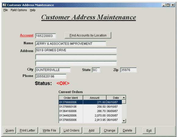
The host program code used to fill the list box is similar to that shown for the error display shown earlier. The program accumulates the order entries into a standard COBOL array then uses the STRING command to stage the ECM LSTDTA command (also see the 4200-LIST-ORDERS section in The Complete COBOL Program). Notice that this command requires that the list box be defined/named in eQuate. In this example, the LST\_ORD multi-column list box is being filled.
