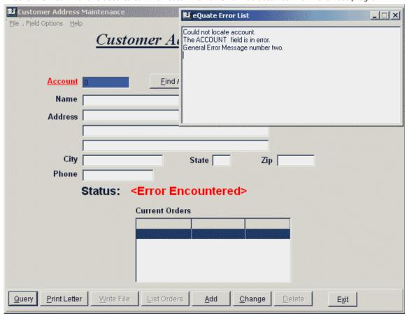
In the example above, the host program has been unable to locate a particular account record and returns an ERRLST command to the eQuate Session Manager causing an independent window titled, "eQuate Error List", to pop up. The host program code used to stage the error with the STRING command is as follows (also see the 4090-Q-INVKEY paragraph in The Complete COBOL Program).
